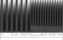
Figure 14. Run 3 conditions with an oxide mask depicting 10μm and 5μm features with a selectivity of 340:1 and an etch rate of 7μm/min
